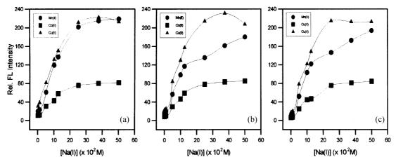
**Figure 6**. Enhanced fluorescence intensities in quenched anthrylazacrown ethers by Mn(II), Co(II) and Cu(II) with the concentration of added sodium nitrate; (a) Anthryl DA15C5, (b) Anthryl MA18C6, (c) Anthryl DA18C6. All solution were mixed with [anthrylazacrown ethers]= $1.0 \times 10^{-7}$  M and [M]= $5.0 \times 10^{-4}$  M. (M=Mn(II), Co(II), Cu(II)). Excitation was at 254 nm and emission maximum centered near 412 nm.
