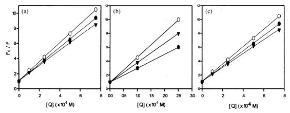
**Figure 4.** Stern-Volmer plotting for anthrylazacrown ethers in quenching with (a) Mn(II), (b) Co(II), and (c) Cu(II). ( $\bullet$ : Anthryl DA15C5,  $\bigcirc$ : Anthryl DA18C6,  $\checkmark$ : Anthryl DA18C6)
