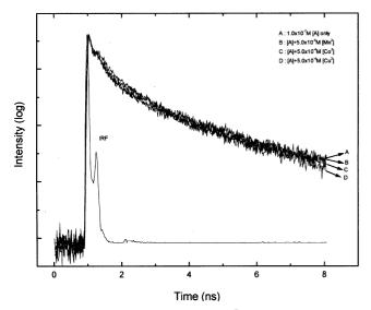
**Figure 5.** TCSPC spectrum of aqueous  $10^{-7}$  M of Anthryl DA15C5 at pH=5 without and with the metal ions Mn<sup>2+</sup>, Co<sup>2+</sup>, and Cu<sup>2+</sup>. The concentration of metal ion is  $5.0 \times 10^{-5}$  M. The excitation wavelength is 300 nm, and the detection wavelength is 410 nm. The notation IRF is the instrumental response function.
