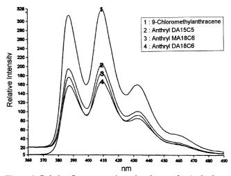
Figure 2. Relative fluorescence intensity changes for Anthrylazacrown ethers in MeOH solution.
