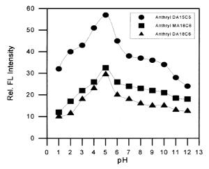
**Figure 3**. pH-fluorescence profiles for 0.1  $\mu$ M solutions of Anthrylazacrown ethers. Excitation was at 254 nm; Emission was measured at the emission maximum centered near 412 nm. pHs were maintained using the following solutions; 0.2 M HCl (pH 1 and 2), 0.2 M Sodium acetate (pH 3, 4, 5 and 6), 0.2 M Tris (pH 7, 8 and 9), 0.2 M NaHCO<sub>3</sub> (pH 10 and 11), 0.2 M NaOH (pH 12).
