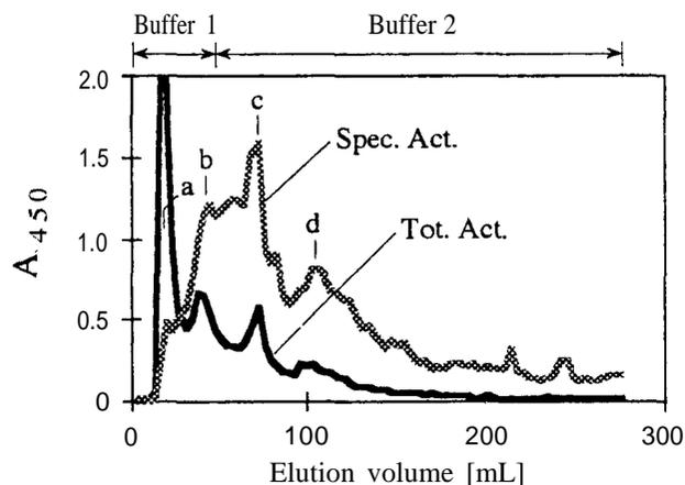
**Figure 1.** Purification of progesterone-glucose oxidase (GO) conjugates by immuno-affinity chromatography. Buffer 1 was a neutral pH buffer, and buffer 2 was an acidic buffer containing Tween. The dark curve represented the total activity (Tot. Act.) of GO and the gray curve the specific activity (Spec. Act.). Peak a contained free GO as major component, and peaks b to d represented different preparations of progesterone-GO conjugates.
