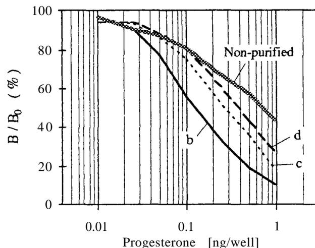
**Figure 2.** Dose-response curves of three affinity-purified progesterone-GO conjugates (b to d from Figure 1) and non-purified GO conjugate mixture. The non-purified mixture required more progesterone to obtain 50% of  $B/B_0$  than did any purified conjugates.
