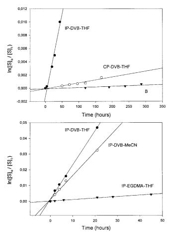
**Figure 1.** Hydrolysis of diphenyl carbonate in 5% HEPES (20 mM, pH 6.8)-MeCN at 15 °C (polymer: 1 mM available cavities, substrate: 5 mM) [top]. Comparison of catalytic performance among imprinted polymers prepared under different conditions in 66% HEPES (0.1 M, pH 7.3)-MeCN at 20 °C (polymer: 2 mM available cavities, substrate: 2 mM) [bottom].
