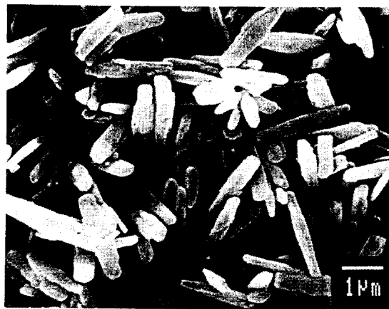
Figure 3. SEM photograph of \text{ZnGa}_2\text{O}_4:\text{Mn} phosphor prepared by the chemical method.
