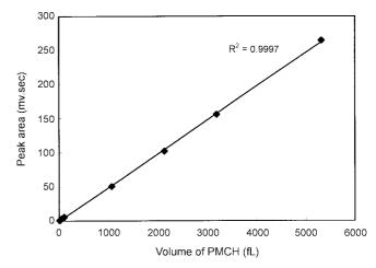
Figure 5. Calibration curve of PMCH standard gas.
