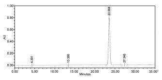
**Figure 4**. HPLC-PDA chromatogram of QN09 (Wavelength 266 nm). Column: Luna C<sub>18</sub>, 4.6 mm × 250 mm, 5  $\mu$ m; mobile phase: MeCN: water: TFA (34 : 66 : 0.1, v:v:v); detector wavelength: 266 nm; flow rate: 1.0 mL/min; Temperature: 30 °C
