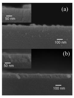
**Figure 4**. SEM images of cross section of post-annealed La<sub>2</sub>CuO<sub>4</sub> thin films at 500 °C (a) and 700 °C (b).
