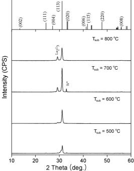
**Figure 1.**  $\theta$ -2 $\theta$ XRD scan of as-deposited La<sub>2</sub>CuO<sub>4</sub> thin films on Si substrate with variation of growing temperature.
