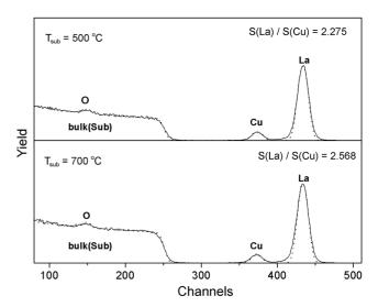
**Figure 2**. Rutherford back scattering (RBS) spectra of as-deposited La<sub>2</sub>CuO<sub>4</sub> thin films on Si substrate.
