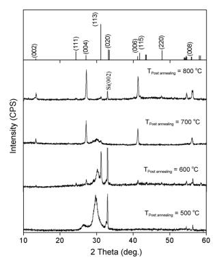
**Figure 3**.  $\theta$ -2 $\theta$  XRD scan of post-annealed La<sub>2</sub>CuO<sub>4</sub> thin films after grown at 500°C on Si substrate.
