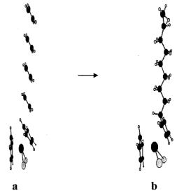
**Figure 11**. Energy minimization process of  $Cp_2TiCl_2 + 4C_2H_4$ . Four ethylenes are arranged oblique to Cp ring keeping the C-C distance between the ethylene carbons 3.0 Å. Structure a is the starting model, and b is an intermediate structure obtained during the optimization.
