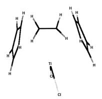
**Figure 10.** The molecular structure of  $Cp_2TiCl_2 + C_2H_4$ . Ethylene is directly combined with the titanium atom through a charge-transfer complex. The bond distances between titanium and two carbon atoms of ethylene are 2.15 Å and 2.15 Å.
