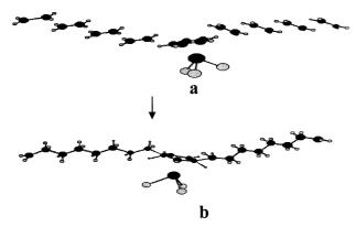
**Figure 8.** Energy minimization process of  $CpTiCl_3 + 8C_2H_4(2-chain)$ . Eight ethylenes in two 4-membered chains are arranged oblique to Cp ring keeping the C-C distance between ethylene carbons 3.0 Å. Structure a is the starting model, and b is an intermediate structure obtained during the optimization.
