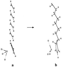
**Figure 7**. Energy minimization process of  $CpTiCl_3 + 4C_2H_4$ . Four ethylenes are arranged oblique to Cp ring keeping the C-C distance between ethylene carbons 3.0 Å. Structure a is the starting model, and b is an intermediate structure obtained during the optimization.
