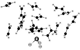
**Figure 3.** Starting model for energy minimization process of CpTiCl<sub>3</sub> + 14C<sub>2</sub>H<sub>4</sub>. Ethylenes are arbitrarily distributed keeping the minimum C-C distance as 3.0 Å
