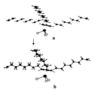
**Figure 9.** Energy minimization process of CpTiCl<sub>3</sub> +  $12C_2H_4(3-chain)$ . Twelve ethylenes in three 4-membered chains are arranged oblique to Cp ring keeping the C-C distance between ethylene carbons 3.0 Å. Structure a is the starting model, and b is an intermediate structure obtained during the optimization.
