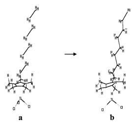
**Figure 15**. Energy minimization process of  $C_{10}H_{15}TiCl_3 + 4C_2H_4$ . Four ethylenes are arranged in a linear chain obliquely and inclined in relation to Cp ring keeping the C-C distance between ethylene carbons 3.0 Å. Structure a is the starting model, and b is an intermediate structure obtained during the optimization.
