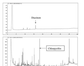
**Figure 7.** Chromatograms of diazinon (0.05 ppm) in pear and chlorpyrifos (1.325 ppm) in perilla leave as determined by GC-NPD or ECD, respectively.
