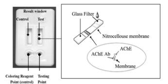
Figure 1. Composition of simple pesticide residue detection strip.
