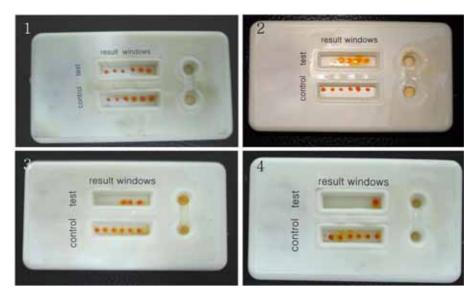
Figure 6. Pesticide residues in real samples 1) diazinon not detected in pear, 2) carrot with diazinon residues of 4.25 ppm, 3) perilla leaves with chlorpyrifos-methyl ranging from 1.25-1.50 ppm, and 4) dropwort with phenthoate at a residue of 4.5 ppm using AChE detection kits.
