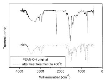
**Figure 6**. IR spectra of *o*-hydroxy polyenaminonitrile (VII); (a) before and (b) after curing reaction.
