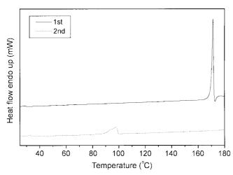
Figure 1. DSC thermograms of compound (III), heating rate 10  $^{\rm o}{\rm C/min}.$
