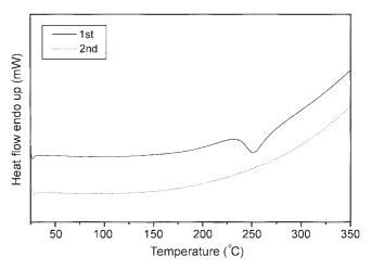
**Figure 4.** DSC thermograms of o-hydroxy polyenaminonitrile (VII).
