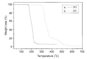
**Figure 2**. TGA thermograms of compound (III, V), heating rate 10 °C/min.
