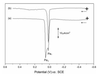
**Figure 2.** Voltammograms of  $Hg(P_{a1})$  and  $Cu(P_{a2})$  at pH 3 by DPASV in (a) 0.1 M KCl and (b) 0.1 M KCl-0.001 M PAR containing 100 ppb Hg and 100 ppb Cu. Deposition time: 240s at -0.5 V vs. SCE. Scan rate: 50 mV/s.
