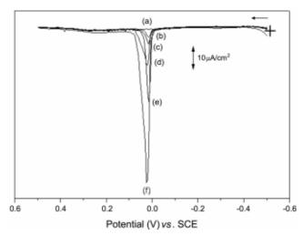
**Figure 4.** Voltammograms of Hg by DPASV in the mixture of Hg and 1000 ppb Cu in 0.1M KCl containing 0.001 M PAR at pH 3. (a) Blank, (b) 10 ppb Hg, (c) 20 ppb Hg, (d) 50 ppb Hg, (e) 100 ppb Hg, and (f) 200 ppb Hg.
