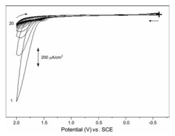
**Figure 1**. Cyclic voltammograms with GC electrode in a solution containing 0.1 M thiophene and 0.1 M quinoline. The potential was cycled 20 times. Scan rate: 50 mV/s. Supporting electrolyte: 0.1 M TBAP in acetonitrile.
