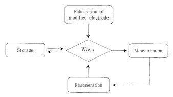
Scheme 1. Block diagram of experimental procedure.
