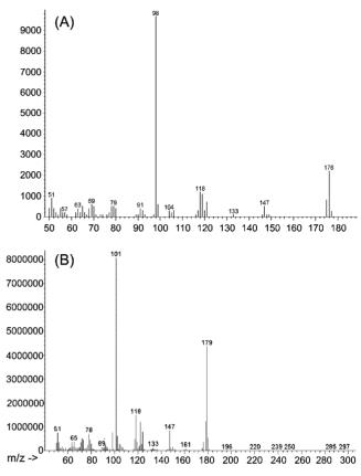
Figure 2. Mass spectra of cotinine (A) and d3-cotinine (B).
