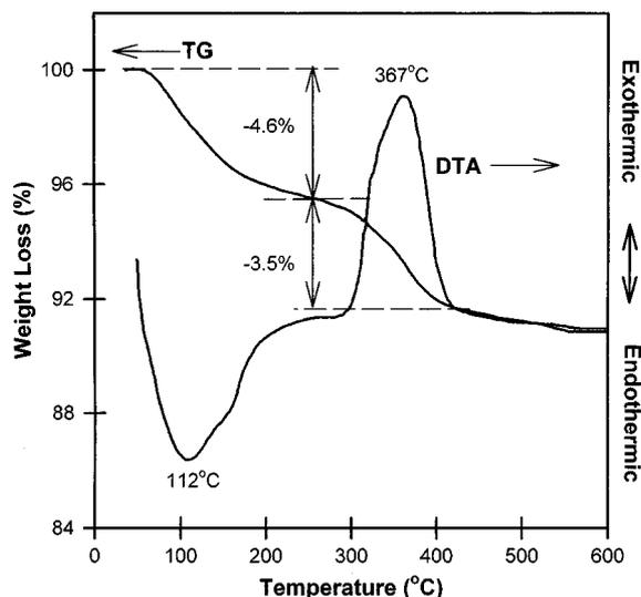
**Figure 3.** TG/DTA results for TCF-pillared clay.
