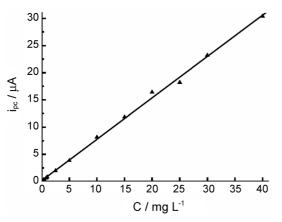
Figure 7. Calibration curve for artemisinin. Accumulation time: 3 min.
