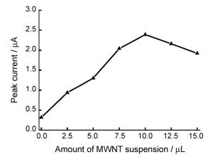
Figure 5. Effect of amount of MWNT/DHP suspension on the reduction peak current of 3.0 mg  $L^{-1}$  artemisinin. Accumulation time: 3 min.
