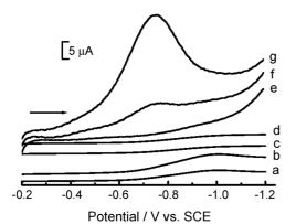
**Figure 4.** LS voltammograms of 30.0 mg L<sup>-1</sup> artemisinin in pH 7.0 phosphate buffer at GCE (a,b); DHP-modified GCE (c,d) and MWNT/DHP modified GCE (f,g). (b,d,g): after 3-min accumulation; (e): blank voltammograms of MWNT/DHP film. Scan rate: 100 mV s<sup>-1</sup>.
