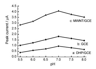
**Figure 3**. Dependence of reduction peak current of 30.0 mg  $L^{-1}$  artemisinin as a function of pH at DHP-modified GCE (a), GCE (b) and MWNT/DHP modified GCE (c).
