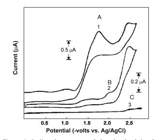
**Figure 6**. Cyclic voltammograms of electrolyzed solution for ABMC. A: after 1st step electrolysis at -1.2 volts, B: after 2nd step electrolysis at -1.8 volts, C: after 3rd electrolysis at -2.3 volts.
