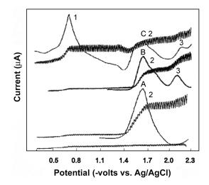
**Figure 2**. Typical DC and DP polarograms of coumarin derivatives in 0.1 M TEAP-AN solution. Scan rate: 50 mV/sec. Current range: 0.02 mA. A:  $1 \times 10^{-3}$  M coumarin, B:  $1 \times 10^{-3}$  M AMC, C:  $5 \times 10^{-4}$  M ABMC.
