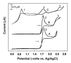
**Figure 3**. Typical cyclic voltammograms of coumarin derivatives in 0.1 M TEAP-AN solution. Scan rate: 50 mV/sec. A:  $1 \times 10^{-3}$  M coumarin, B:  $1 \times 10^{-3}$  M AMC, C:  $5 \times 10^{-4}$  M ABMC.
