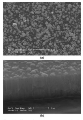
Figure 5. SEM images of a plan view (a) and a prospective view (b) of an CdS/Co nanowire array deposited in an AAO template.
