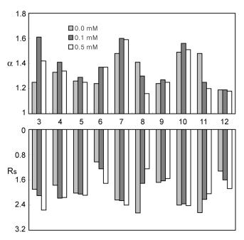
Figure 4. The trends of the separation (a) and the resolution factors (R<sub>S</sub>) for the resolution of  $\beta$ -amino acids 3-12 on CSP 2 with the variation of the ammonium acetate (NH<sub>4</sub>OAc) concentration (0.0 mM, 0.1 mM and 0.5 mM) in aqueous mobile phase.
