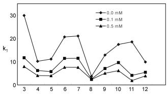
**Figure 3**. The trends of the retention factors  $(k_1)$  for the resolution of  $\beta$ -amino acids **3-12** on CSP **2** with the variation of the ammonium acetate (NH<sub>4</sub>OAc) concentration (0.0 mM, 0.1 mM and 0.5 mM) in aqueous mobile phase.
