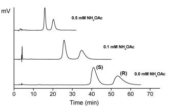
**Figure 5**. The representative chromatograms for the resolution of 3-amino-4-(4-methylphenyl)butyric acid (4) on CSP 2 with the variation of the ammonium acetate (NH<sub>4</sub>OAc) concentration (0.0 mM, 0.1 mM and 0.5 mM) in aqueous mobile phase. For the chromatographic condition, see the foot note to Table 2.
