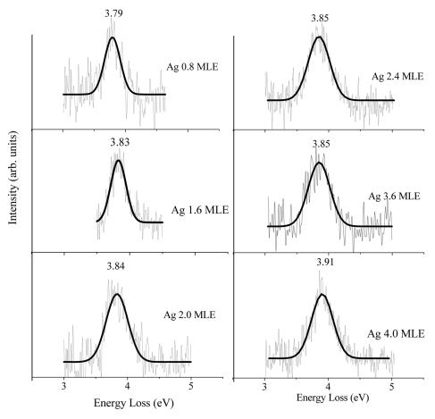
**Figure 5.** HREELS spectra for Ag particles grown on mildly sputtered HOPG surfaces. (Ag coverages below 4 monolayers equivalent (MLE)) An exponentially decaying background was subtracted from each spectrum. For these spectra, the best fits can be achieved using a single Gaussian function, indicating the disappearance of the interband and intraband transition with decreasing particle size
