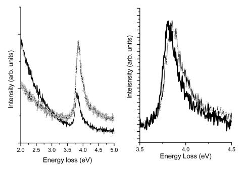
Figure 4. HREELS spectra of Ag on HOPG before (dot + line) and after heating (line) to about 400 K. A narrowing of the peak width and a shift to lower binding energy is observed upon heating the sample to 400 K. Left: raw data Right: After subtracting background and normalization.
