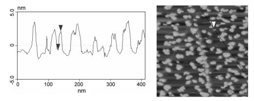
Figure 3. AFM image and a height profile of Ag particles on HOPG. About 4 MLE of Ag was deposited on HOPG.
