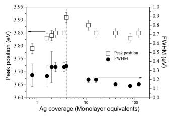
**Figure 6**. Variations of the peak position and width for the Ag plasmon resonance as a function of Ag coverage.
