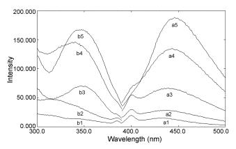
Figure 3. Emission and excitation spectra: al & b1 Emission and excitation of reagents blank; a2 & b2: Emission and excitation of urine blank; a3 & b3: Emission and excitation of MF after administration of MF to volunteer and CPE of MF from urine; a4 & b4: Emission and excitation of MF spiked to the urine; a5 & b5: Emission and excitation of MF standard solution (1.0 mg L<sup>-1</sup>); 0.05 mol L<sup>-1</sup> HCl; 0.1% Triton X-114.
