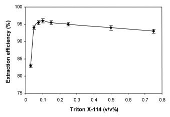
Figure 5. Effect of Triton X-114 concentration on the extraction efficiency:  $1.0 \text{ mg L}^{-1} \text{ MF}$ ; 0.05 mol L<sup>-1</sup> HCl.
