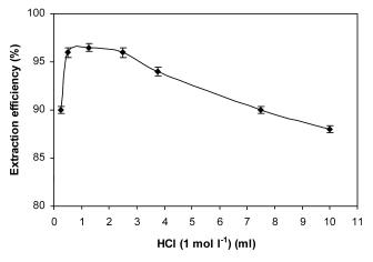
Figure 4. Effect of HCl concentration on the extraction efficiency:  $1.0 \text{ mg L}^{-1} \text{ MF}$ ; 0.1% Triton X-114.
