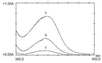
**Figure 2**. Absorption spectra of MF: a) standard solution (1.0 mg  $L^{-1}$ ); b) extracted from spiked urine; c) extracted from urine after administration to volunteer. 0.05 mol  $L^{-1}$  HCl, 0.1% Triton X-114.
