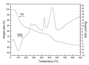
Figure 2. TG and DTA plots of the dried gel recorded between 30 and 900  $^{\circ}$ C at a heating rate of 5  $^{\circ}$ C/min.
