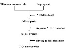
Figure 1. Process for synthesis of TiO<sub>2</sub> nanopowder.
