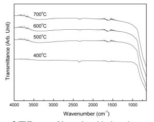
Figure 5. FT-IR spectra of the powders calcined at various temperatures between 400  $^{\circ}$ C and 700  $^{\circ}$ C.
