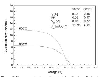
**Figure 8**. Photocurrent-voltage characteristics of solar cells developed by using TiO<sub>2</sub> powders synthesized by the sol-gel combustion hybrid method at 500 °C and 600 °C. The measurement was carried out at room temperature with a light intensity of 100 mW/cm<sup>2</sup>, spectral irradiance of AM 1.5, and an active cell area of 0.25 cm<sup>2</sup>.
