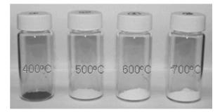
Figure 3. Colours of the powders calcined at various temperatures between 400 and 700  $^{\circ}$ C.
