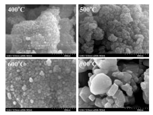
Figure 7. SEM images of the powders calcined at various temperatures between 400 and 700 °C.
