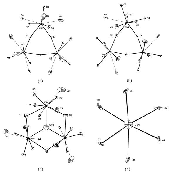
Figure 3. Labeled diagrams of CaO<sub>n</sub> polyhedron in the unit cell. (a) Ca(1)O<sub>8</sub>, (b) Ca(2)O<sub>8</sub>, (c) Ca(3)O<sub>9</sub>, (d) Ca(4)O<sub>6</sub>
