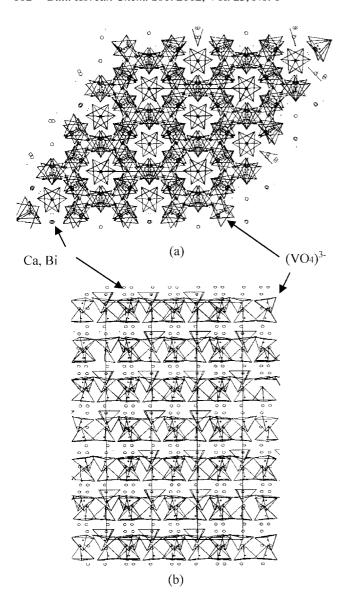
**Figure 5**. ORTEP diagrams of the unit cell on the  $Ca_{1.29}Bi_{0.14}VO_4$  crystal. (a) unit cell looking down the c-axis. (b) unit cell looking down the a-axis.
