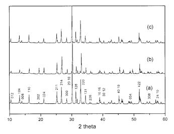
**Figure 2**. (a) XRD pattern of Ca<sub>1.29</sub>Bi<sub>0.14</sub>VO<sub>4</sub> composition sintered for 72hr at 1100 °C. (b) XRD pattern of pale yellow crystals grown at a rate of 2 °C/hr. (c) XRD pattern of the yellow crystals grown at a rate of 2 °C/hr.
