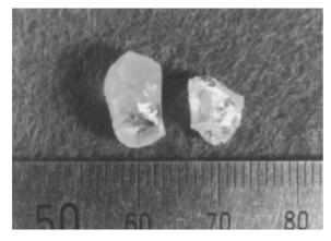
**Figure 1**. Photographs of the crystals grown at the cooling rate of 2 °C/hr.
