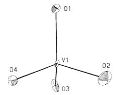
Figure 4. Labeled diagram of  $(VO_4)^{3-}$  tetrahedron in the unit cell.
