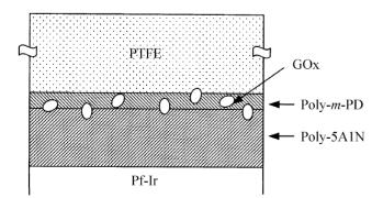
**Figure 1**. Schematic view of the trilayered glucose sensor. The thicknesses of poly-5A1N, poly-*m*-PD and PTFE are *ca*. 24 nm, 8 nm and 4  $\mu$ m, respectively.
