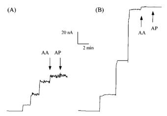
**Figure 2.** The current responses of Pt-Ir\poly-5A1N\poly-*m*-PD+GOx (A) and Pt-Ir\poly-5A1N\poly-*m*-PD+GOx\PTFE (B) to 6 mM glucose, 0.11 mM AA and 0.17 mM AP in PBS. The concentrations of AA and AP are the physiological maximum.
