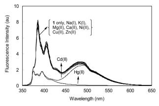
**Figure 1.** Fluorescence spectra of **1** in the presence of various metal ions. [1] =  $5.0 \times 10^{-6}$  M, [ $M^{n+}$ ] =  $5.0 \times 10^{-4}$  M in aqueous acetonitrile solution ( $H_2O:CH_3CN = 50:50$ , v/v) buffered at pH 8.1 (10 mM of Tris).  $\lambda_{ex} = 340$  nm. The pH value denotes that of water portion before mixing with acetonitrile.
