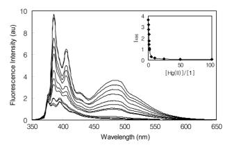
**Figure 3**. Fluorescence titration of **1** with Hg<sup>2+</sup> ions in aqueous acetonitrile (H<sub>2</sub>O:CH<sub>3</sub>CN = 50:50, v/v). [**1**] =  $5.0 \times 10^{-6}$  M.  $\lambda_{\rm ex}$  = 340 nm. In buffered solution at pH 8.1 (10 mM of Tris).
