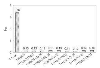
**Figure 4**. Changes in the fluorescence intensity of **1** at 486 nm in response to the Hg<sup>2+</sup> ions in the presence of various coexistent metal ions. [**1**] =  $5.0 \times 10^{-6}$  M, [M<sup>n+</sup>] =  $5.0 \times 10^{-4}$  M, [Hg<sup>2+</sup>] =  $5.0 \times 10^{-5}$  M, in aqueous acetonitrile solution (H<sub>2</sub>O:CH<sub>3</sub>CN = 50:50, v/v) buffered at pH 8.1 (10 mM of Tris).  $\lambda_{ex}$  = 340 nm.
