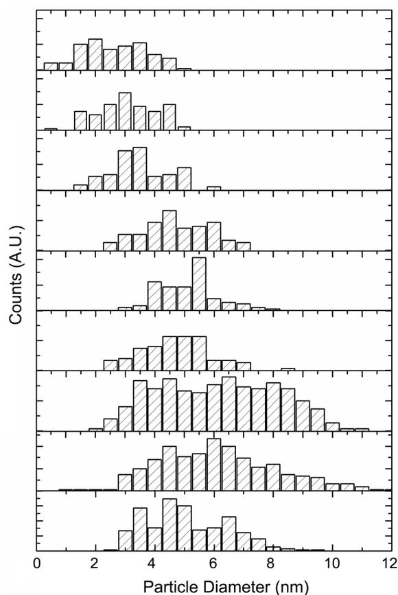
**Figure 2.** Histograms of particle sizes obtained from TEM images of holding-at-250mV-20, R- $^{13}\text{C}$ CO-20, R-CO-20, holding-at-250mV-40, R- $^{13}\text{C}$ CO-40, R-CO-40, holding-at-250mV-60, R- $^{13}\text{C}$ CO-60, and R-CO-60 sample from top to bottom.
