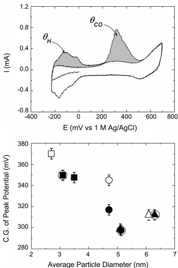
**Figure 3.** The CO stripping CV of a holding-at-250mV-20 sample (top) and a plot of center of gravity of CO oxidation peak potential of CO stripping CV versus average Pt particle size measured by TEM (bottom). Square, circle, and triangle shapes represent 20, 40, and 60% Pt/C sample data, respectively. Filled shapes are used for R-CO-X data whereas additional outer circle is added to the filled shape to denote R-<sup>13</sup>CO-X data.
