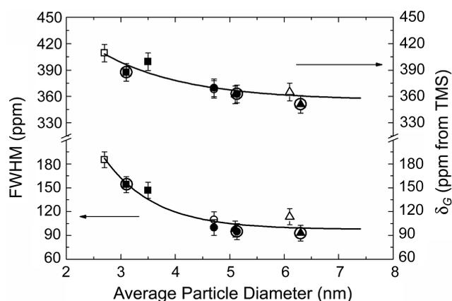
**Figure 5.** The full width at half height (FWHM) and the center of gravity ( $\delta_G$ ) plot of the <sup>13</sup>CO NMR spectra with respect to average particle size taken from our TEM results: Square, circle, and triangle shapes represent 20, 40, and 60% Pt/C sample data, respectively. Filled shapes are used for R-CO-X data whereas additional outer circle is added to the filled shape to denote R-<sup>13</sup>CO-X data.
