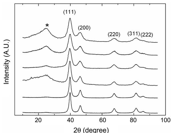
**Figure 1.** Powder XRD patterns of holding-at-250mV-20, R-CO-20, holding-at-250mV-40, R-CO-40, holding-at-250mV-60 and R-CO-60 sample from top to bottom. Miller index of each diffraction signal is denoted on the top of the signal and broad carbon background signal is marked by \*.
