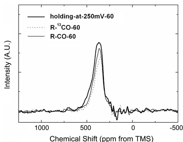
**Figure 4.** The <sup>13</sup>C NMR spectra of adsorbed <sup>13</sup>CO on 60% Pt supported on carbon samples after subtracting the carbon graphite signal.
