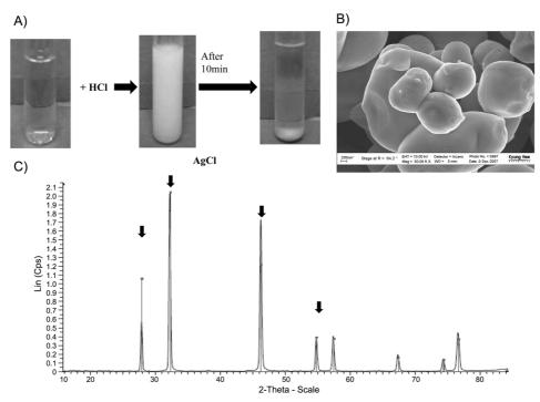
**Figure 2.** The property of nanometer sized silver materials. The process for the formation of the nano silver precipitate is shown in (A). The FE-SEM analysis of the precipitate (B); the X-RD pattern of the precipitate (C). The sediment analysis yielded AgCl by X-RD, which suggests the presence of Ag ions in the nanometer the silver solutions.
