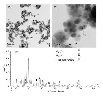
**Figure 1.** HRTEM images of nanometer sized silver are shown in (A) and (B). The nano-silver sol (A), and extension images (B). The X-RD pattern is shown in (C). There are several compounds  $(Ag_3O, Ag_3H)$  and titanium oxide) in the nanometer sized silver material
