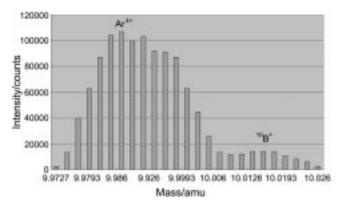
**Figure 1**. Mass spectrum showing slight overlapping of <sup>40</sup>Ar<sup>4+</sup> peak onto <sup>10</sup>B<sup>+</sup> peak.
