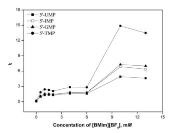
**Figure 1**. Retention factors (k) of nucleotides without and with  $[BMIm][BF_4]$  in mobile phase.
