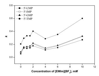
**Figure 3**. Retention factors (k) of nucleotides without and with  $[EMIm][BF_4]$  in mobile phase.
