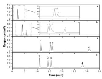
**Figure 2.** Chromatograms of a mixture of nucleotides with mobile phases without (a) and with 0.5 (b), 10.0 (c) and 13.0 (d) m*M* [BMIm][BF<sub>4</sub>] (peaks numbering: (1) 5'-UMP, (2) 5'-IMP, (3) 5'-GMP, (4) 5'-TMP).
