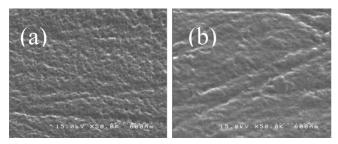
**Figure 2.** The SEM image of the surface of the GC after the preanodization (a) and polymerization (b), respectively.
