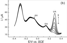
**Figure 4.** (a) DPV of DA with different concentrations (a-i: 0, 2, 4, 6, 10, 20, 30, 50, 70  $\mu$ M) at a PTGCE in the presence of 500  $\mu$ M AA and 15  $\mu$ M UA (b) DPV of UA with different concentrations (a-g: 2, 6, 10, 15, 25, 45, 75  $\mu$ M) at PTGCE in the presence of 500  $\mu$ M AA and 15  $\mu$ M DA.
