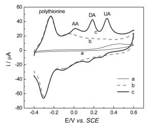
**Figure 3**. CVs for a mixture of 500  $\mu$ M AA, 20  $\mu$ M DA and 100  $\mu$ M UA in pH 6.5 PBS at GCE (a) and PTGCE (c). CV for PTGCE in the blank solution (b).
