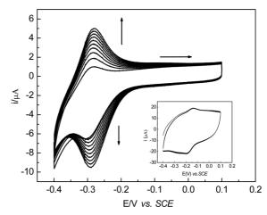
**Figure 1**. CVs for the electropolymerization of thionine on preanodizd GC in 0.1 M PBS (pH 6.5). The inset shows CV for pure GC. scan rate:  $0.1~\rm Vs^{-1}$ .
