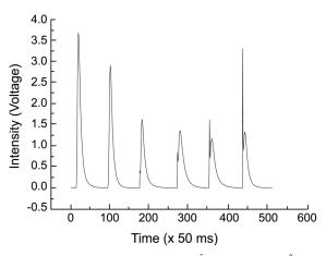
**Figure 6**. Peaks of epinephrine  $(1 \times 10^{-5} \text{ g/mL})$  when Fe<sup>3+</sup> ions of 0, 1, 2.5, 5, 10, and 20 µg/mL were added in turn.
