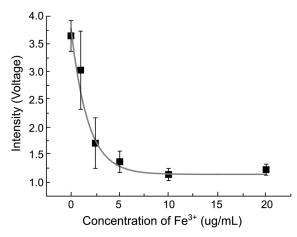
**Figure 7**. Interference effect of Fe<sup>3+</sup> ion on the integrated peak area of epinephrine; PMT 600 V, op amp  $10^5$ , 0.01 M luminol (in phosphate buffer), 0.01 M NaIO<sub>4</sub>, epinephrine  $(1 \times 10^{-6} \text{ g/mL})$ .
