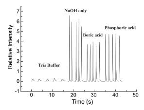
Figure 2. Effect of buffer on chemiluminescence reaction; PMT 450 V, op amp  $10^5$ , 0.01 M luminol (in 0.1 M buffers), 0.01 M NaIO<sub>4</sub>, Epinephrine  $1 \times 10^{-5}$  g/mL.
