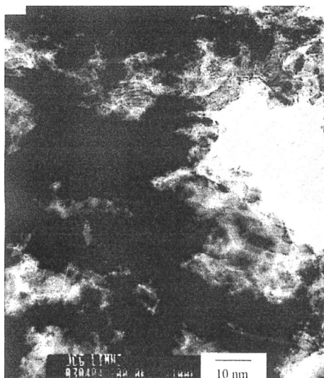
Figure 11. TEM micrograph of nanocrystalline 'LiMn 2 O 4 '. The average crystallite size is ~50 Å.
