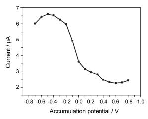
**Figure 10**. Influence of accumulation potential on the oxidation peak current of  $1.0 \times 10^{-5}$  mol L<sup>-1</sup> acetaminophen in phosphate buffer (pH 5.0). Accumulation time: 80 s.
