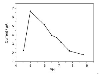
**Figure 8**. Dependence of the oxidation peak current of  $1.0 \times 10^{-5}$  mol L<sup>-1</sup> acetaminophen on the pH value. Supporting electrolyte: 1/15 mol L<sup>-1</sup> phosphate buffer.
