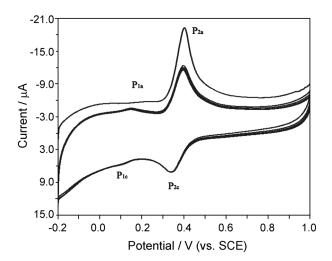
**Figure 2.** Cyclic voltammograms of  $1.0 \times 10^{-5}$  mol L<sup>-1</sup> acetaminophen at the MWNT/DHP/PEG composite film electrode in phosphate buffer (pH = 5.0). Scan rate:  $100 \text{ mV s}^{-1}$ .
