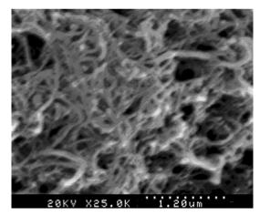
Figure 1. Scanning electronic microscopy image of MWNT/DHP/ PEG composite film electrode.
