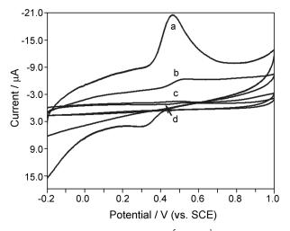
**Figure 3**. Voltammograms of  $1.0 \times 10^{-5}$  mol L<sup>-1</sup> acetaminophen at (a) the MWNT/DHP/PEG composite film electrode; (b) the DHP/PEG film electrode; (c) the unmodified electrode and (d) the DHP film electrode in phosphate buffer (pH = 5.0). Scan rate: 100 mVs<sup>-1</sup>.
