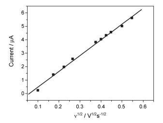
Figure 5. Dependence of the oxidation peak current on the scan rate.
