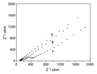
**Figure 7**. Nyquist diagram (Z' vs. Z") for the MWNT/DHP/PEG film electrode (a), the MWNT/DHP film electrode (b) and the unmodified electrode (c) in the presence of 10 mmol  $L^{-1}$  K<sub>3</sub>[Fe(CN)<sub>6</sub>]/K<sub>4</sub>[Fe(CN)<sub>6</sub>](1:1)-mixture. 0.2 mol  $L^{-1}$  KCl was used as supporting electrolyte.
