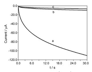
**Figure 6**. Chronocoulometry of  $1.0 \times 10^{-4}$  mol L<sup>-1</sup> acetaminophen at the MWNT/DHP/PEG composite film electrode (a), the unmodified electrode (b) and the DHP film electrode(c). Initial potential 0.60 V, final potential 1.00 V, and pulse width 30 s.
