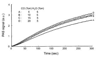
Figure 5.  $P_{H_2O}$  dependence of CO<sub>2</sub> photoacoustic signal for the water-gas shift reaction over magnetite/chromium oxide catalyst at 300 °C.
