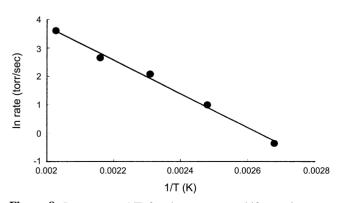
Figure 8. Ln rate vs. 1/T for the water-gas shift reaction over copper/zinc oxide catalyst.
