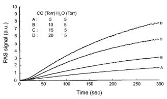
Figure 4.  $P_{CO}$  dependence of CO<sub>2</sub> photoacoustic signal for the water-gas shift reaction over magnetite/chromium oxide catalyst at 300 °C.
