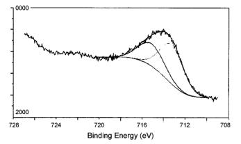
Figure 6. Fe(2p<sub>3/2</sub>) XPS spectrum of the vacuum-treated magnetite/ chromium oxide catalyst.
