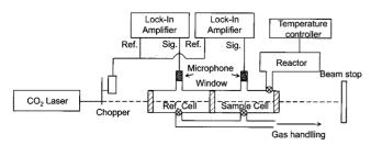
Figure 1. An experimental setup for the photoacoustic detection method.
