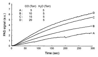
Figure 9. P<sub>CO</sub> dependence of CO<sub>2</sub> photoacoustic signal for the water-gas shift reaction over copper/zinc oxide catalyst at 200 °C.
