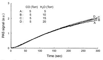
Figure 10.  $P_{H_2O}$  dependence of CO<sub>2</sub> photoacoustic signal for the water-gas shift reaction over copper/zinc oxide catalyst at 200 °C.
