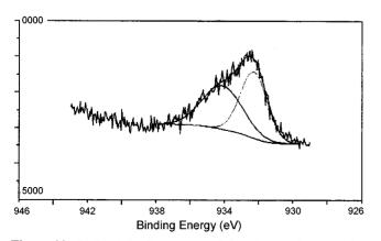
Figure 11.  $Cu(2p_{3/2})$  XPS spectrum of the H<sub>2</sub>-treated copper/zinc oxide catalyst.
