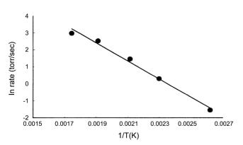
Figure 3. Ln rate vs. 1/T for the water-gas shift reaction over magnetite/chromium oxide catalyst.
