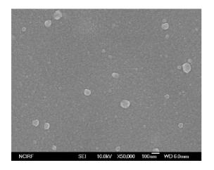
Figure 2. FE-SEM image of naproxen-loaded PEO-b-PMAA micelle.
