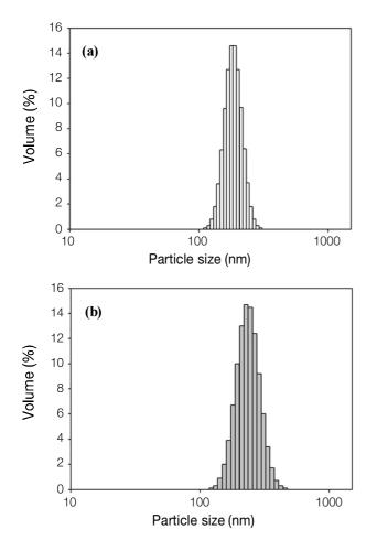
**Figure 1.** Size distribution of (a) PEO-*b*-PMAA micelle, and (b) naproxen-loaded PEO-*b*-PMAA micelle.
