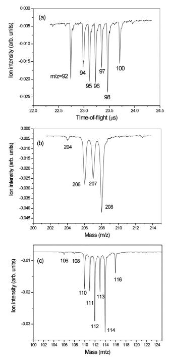
**Figure 5.** Laser ablation/ionization TOF-MS spectra for molybdenum (5-a), lead (5-b) and cadmium (5-c). The laser energy is  $2.5 \, \text{mJ/pulse}$  and the size of laser beam at the sample surface is  $2 \, \text{mm}^2$ .
