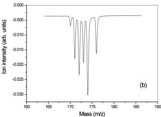
**Figure 6**. Mass spectra of Yb coated on the stainless steel substrate. Figure 7-(a) shows ion signals generated from the stainless steel, while Figure 7-(b) shows well-resolved mass spectrum of ytterbium. The laser energy is adjusted as to 1.2 mJ/pulse in both spectra.
