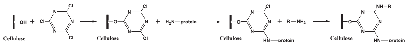
Figure 1. Schematic diagram for the activation of cellulose by cyanuric chloride and immobilization of HpAOD by covalent linkage.
