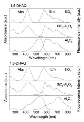
**Figure 1**. Absorption and fluorescence spectra of 1,5-DHAQ (upper) and 1,8-DHAQ (bottom) in SiO<sub>2</sub>, SiO<sub>2</sub>-Al<sub>2</sub>O<sub>3</sub> (sample C in Table 1) and Al<sub>2</sub>O<sub>3</sub> matrices, respectively.
