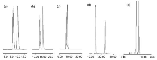
**Figure 2**. Chiral separation of 2,2,2-trifluoro-1-(9-anthryl)ethanol on CSP 1(a), CSP 2(b), CSP 3(c), CSP 4(d), and CSP 5(e). Eluent: 10% IPA/hexane, flow rate: 1.5 mL/mim, UV 254 nm.
