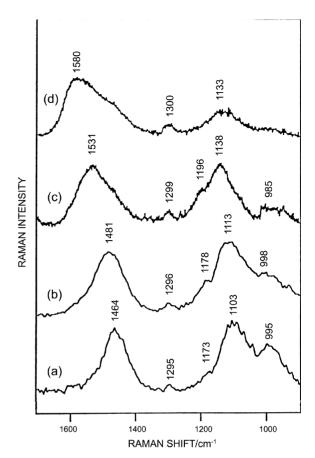
**Figure 3**. Resonance Raman spectra of HClO<sub>4</sub>-doped *trans*-PA. Excitation wavenumbers are 1320-, 1064-, 753-, and 514.5-nm for (a), (b), (c), and (d), respectively. The dopant content of HClO<sub>4</sub> is 8 %. Fluorescence backgrounds are subtracted from each spectrum.
