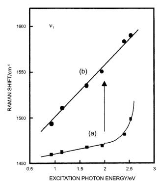
**Figure 4.** Plot of the Raman wavenumbers ( $v_1$  band) versus the excitation photon energies (2.54-0.94 eV): (a) Pristine *trans*-PA and (b) Na-doped *trans*-PA.
