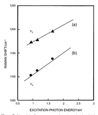
Figure 7. Plot of the Raman wavenumbers ( $v_3$  and  $v_4$  bands) for HClO<sub>4</sub>-doped trans-PA against the excitation photon energies (2.54-0.94 eV): (a)  $v_3$  and (b)  $v_4$  bands.
