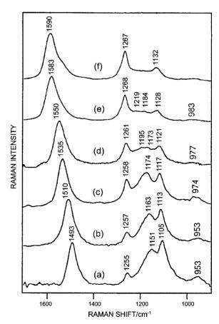
**Figure 2**. Resonance Raman spectra of heavily Na-doped *trans*-PA. Excitation wavenumbers are 1320-, 1064-, 753-, 632.8-, 514.5-, and 488-nm for (a), (b), (c), (d), (e), and (f), respectively. The dopant content of Na is above 15 mol %. Fluorescence backgrounds are subtracted from each spectrum.
