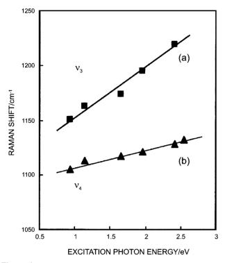
**Figure 6**. Plot of the Raman wavenumbers ( $v_3$  and  $v_4$  bands) for Na-doped trans-PA against the excitation photon energies (2.54-0.94 eV): (a)  $v_3$  and (b)  $v_4$  bands.
