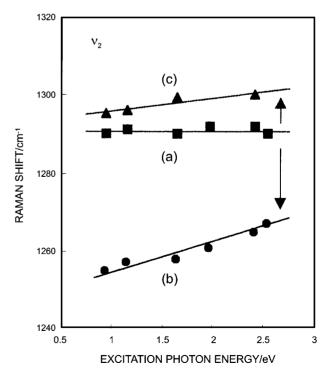
**Figure 5**. Plot of the Raman wavenumbers ( $v_2$  band) versus the excitation photon energies (2.54-0.94 eV): (a) Pristine *trans*-PA, (b) Na-doped *trans*-PA, and (c) HClO<sub>4</sub>-doped *trans*-PA.
