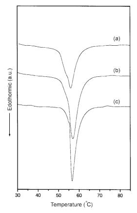
**Figure 3.** DSC thermograms of hydrated bilayers in PBS (about 50 wt%) of (a) DSPC only, (b) DSPC/PEG-Phe-Chol (95/5), and (c) DSPC/PEG-Phe-Chol (90/10). All of the thermograms were obtained from the second heating scans and the scan rate was 5 °C/min
