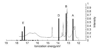
**Figure 1**. The theoretical ionization spectrum of OsO<sub>4</sub> calculated by non-relativistic CASPT2.
