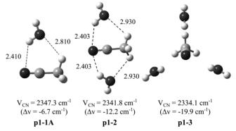
**Figure 3**. The structures of  $(CH_3CN)$ - $(H_2O)_n$  (n = 1-3) clusters with increasing  $\pi$ -type bonding character.
