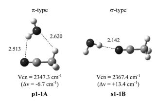
Figure 1. The structures and C-N stretching harmonic frequencies of (CH<sub>3</sub>CN)-(H<sub>2</sub>O) complexes.
