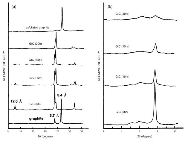
Figure 3. X-ray diffraction patterns of the SO<sub>3</sub> intercalated graphite at various reaction times: (a)  $2\theta$ : 5-35, (b)  $\theta$ : 2-10.
