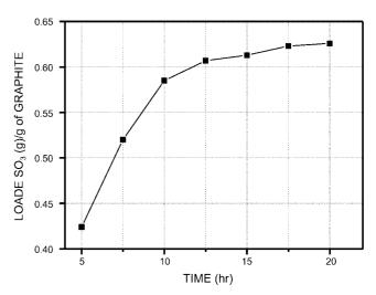
Figure 2. Loaded SO<sub>3</sub> gas per g-graphite depending on the reaction time.
