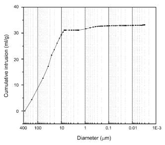
**Figure 6**. Pore characteristic of the exfoliated graphite by the mercury porosimetry.
