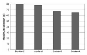
**Figure 8**. Maximum sorption capacity of the exfoliated graphite for different grade heavy oil.
