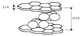
**Figure 4**. Schematic draws for the hypothetical configuration of  $SO_3$  molecules in the graphite interlayer.
