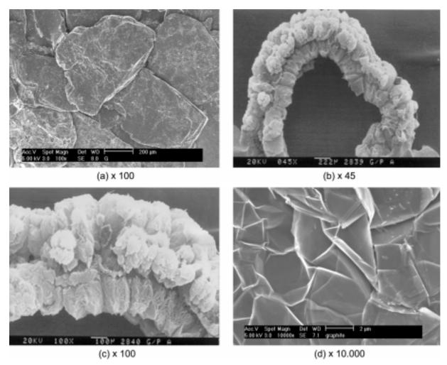
Figure 7. SEM (scanning electron micrographs) for exfoliated graphite.
