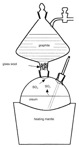
**Figure 1**. Reaction equipment for the reaction between graphite and  $SO_3$  gas.
