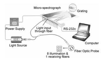
Figure 1. The schematic diagram of the miniaturized spectrometer.
