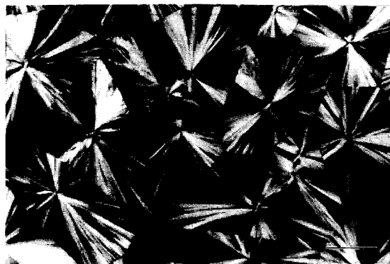
Figure 4. A polarizing optical micrograph (43 \mu\text{m} scale bar) of PTMS spherulites grown at 90 °C.
