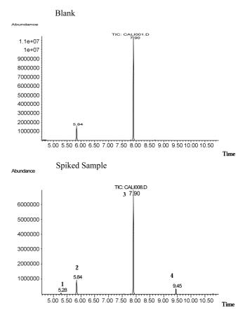
**Figure 1**. Chromatograms of the extracts from milli-Q water (blank) and milli-Q water spiked with 80 ng/mL of standards. (1=EGME, 2=EGEE, 3=EGBE, 4=DEGME).
