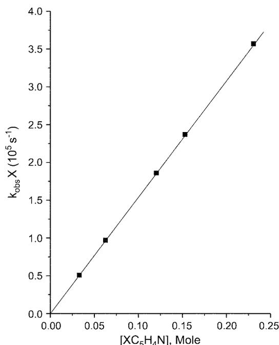
**Figure 4.** Plots of pseudo-first order rate constants ( $k_{obs}$ ) vs. nucleophile concentration,  $[XC_5H_4N]$ , for reaction of *m*-cyanoaryl cyclopropanecarboxylate with X-pyridine (X=H) in acetonitrile at 55.0 °C.
