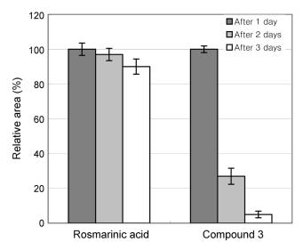
**Figure 3**. The stability of the compounds in buffer solution. Sample solution (100  $\mu$ g/mL) was incubated at 37 °C buffer solution (pH 7.4). The initial time was recorded and 100  $\mu$ g/mL of the solution was removed at known time intervals and was analyzed by reverse-phase HPLC.
