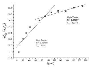
Figure 4. Plot for gas kinetic temperature measurement using OH spectrum.
