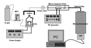
**Figure 1**. Schematic diagram of ETV-microchip plasma (ETV-MCP) system.
