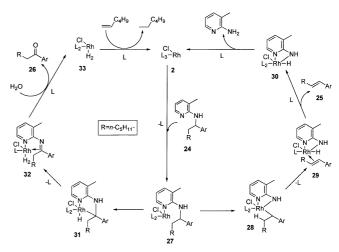
**Scheme 3.** Catalytic Cycle for the Carbon-Nitrogen Bond Cleavage and Dehydrogenation (L=PPh<sub>3</sub>).
