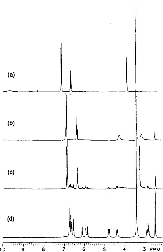
Figure 3. ^1\text{H} NMR spectra of 1 in the presence of LiOD in DMSO- d_6 . (a) without base, (b) 1 equivalent of LiOD, (c) 2 equivalents of LiOD, (d) 3 or more equivalents of LiOD.
